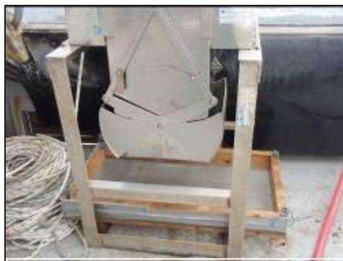
(a) Box core used to collect sediment and biota samples.
