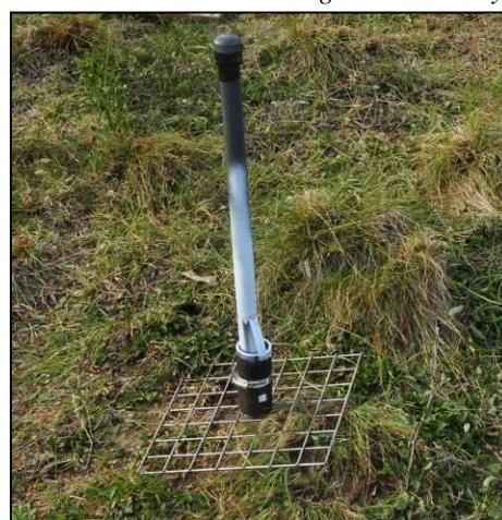
*A completed frost tube including a screen to measure frost heave, Ramah Bay*
