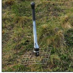
A completed frost tube including a screen to measure frost heave, Ramah Bay
