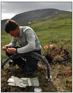
Angus Simpson bear-proofing the temperature cable near Ivitak Cove. The cable will record soil temperature to a depth of 7 m every 6 hours all year long.
