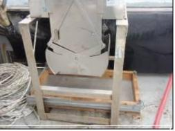
(a) Box core used to collect sediment and biota samples.
