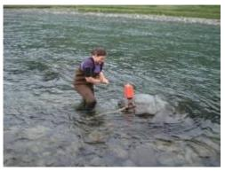
Deploying a pressure sensor in Nachvak Brook
